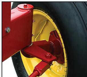
**CR Spindles** and greasable hubs are standard on all wheels.
