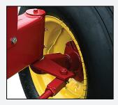
**CR Spindles** and greasable hubs are standard on all wheels.
