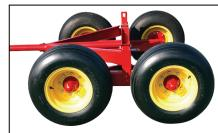
**Tandem axle models** feature a **Walking Beam** that is offset 2" toward the rear axle. Because this throws a little more weight on the rear axle, the front axle enters holes and ditches more smoothly. The offset walking beam creates greater stability and a better ride over uneven ground.
