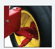
**CR Spindles** and greasable hubs are standard on all wagon gears.
