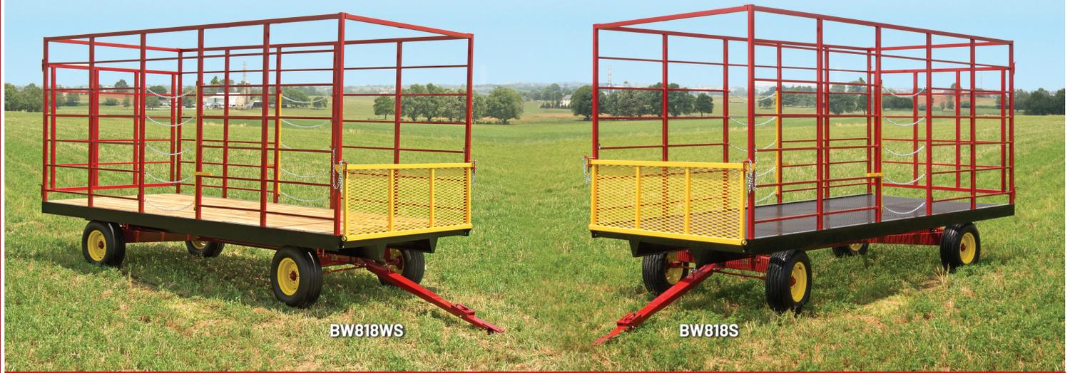
Farmco bale wagons provide generous size, weight, and smooth handling. They have been used on farms for over 20 years. Boxes come in 8' or 9' widths and 18' and 22' lengths. Most models are fabricated with an all-steel frame using 7" channel main beams and formed steel cross pieces.
