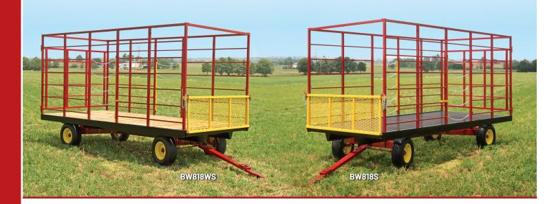
Farmco bale wagons provide generous size, weight, and smooth handling. They have been used on farms for over 20 years. Boxes come in 8' or 9' widths and 18' and 22' lengths. Most models are fabricated with an all-steel frame using 7" channel main beams and formed steel cross pieces.
