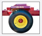
**Cold-rolled axle spindles** and greasable hubs on all wheels.
