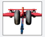
**180-degree front turning dolly** and **extendable tongue** for easy hookup and variable towing lengths.
